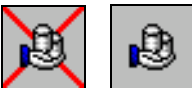
Figure 20. The icons showing the status of the socket connection with the Oracle database. Left icon corresponds to no connection to the database. Right icon is used when the connection to the Oracle database is open.
