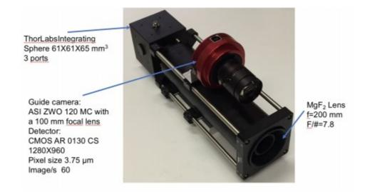
Figure 3. The LOCNES telescope.
